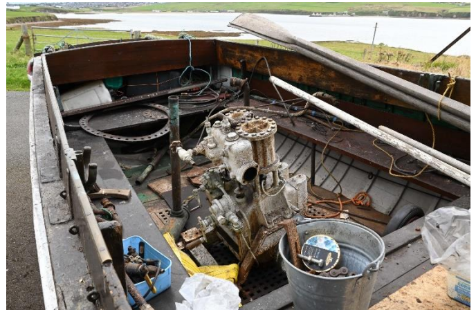
Figure 20- the steam engine used to drive Nellie
