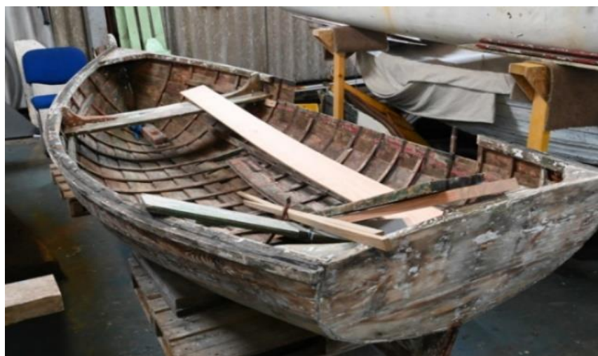
Figure 43- Paint scraped and all rotten boards and timbers removed
