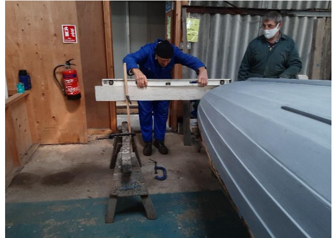
Figure 40- Similarly erect a horizontal board at transom where you want the line to be.
