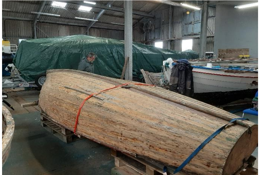
Figure 35 - Paint stripped and drying out, ready for painting.
