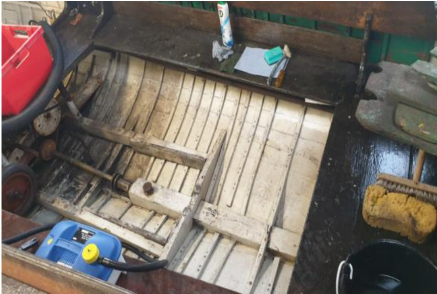
Figure 46 - Inside of hull being cleaned with a steam cleaner
