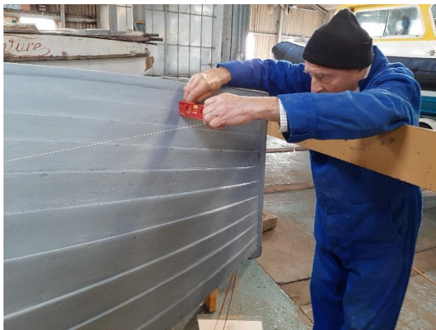
Figure 40- String a line from front board to aft board to be as close to the hull as possible. Transfer marks level with line onto hull every 150mm or so.
