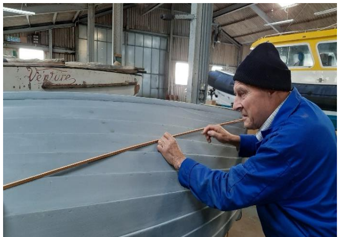
Figure 40 - Draw a fair line using the marks with a triangular section thin batten.
