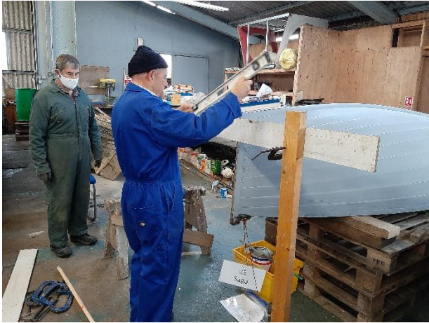
Figure 40 - Set up horizontal board at bow where line to be.
