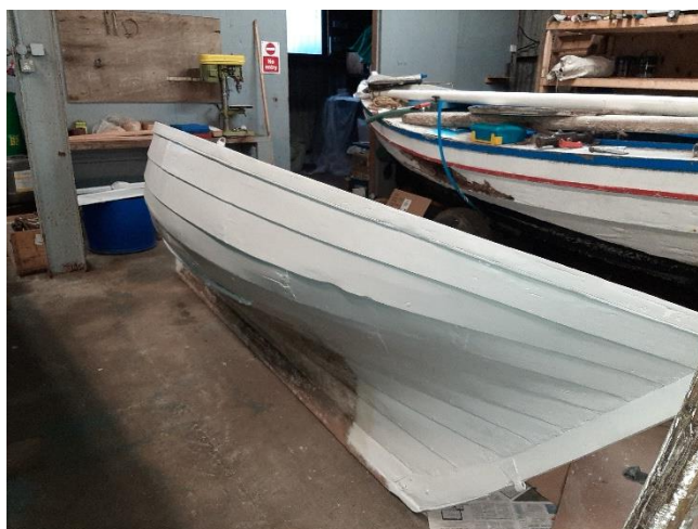
Figure 42 - Painting the hull with primer in progress
